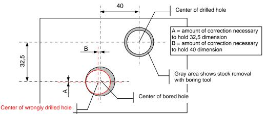
In the illustration, the original drilled hole is out of print tolerance. In other words, the centerline distance between the holes is not correct. By simply dialing in the correct centerline distance the hole can be re-bored to its true position. However, this operation can only be successful if there is sufficient stock remaining in the hole for a 100% cleanup.
