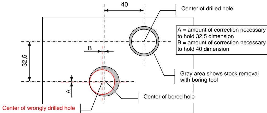
In the illustration, the original drilled hole is out of print tolerance. In other words, the centerline distance between the holes is not correct. By simply dialing in the correct centerline distance the hole can be re-bored to its true position. However, this operation can only be successful if there is sufficient stock remaining in the hole for a 100% cleanup.
